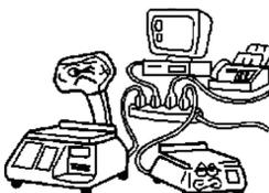
Sharing sockets with other high-power devices can cause large fluctuations. Make sure that one scale uses a matching power outlet.
