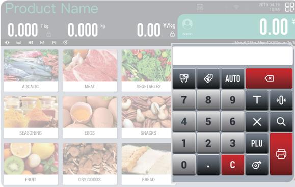
The numeric keyboard can be used to call up functions such as merchandise, promotion, peeling, zero setting, paper feeding, printing and so on.
