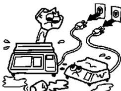
Immediately turn off the switch and Plug when metal fragments or liquids enter the interior, suspend use and contact service personnel to avoid fire or electric shock.
